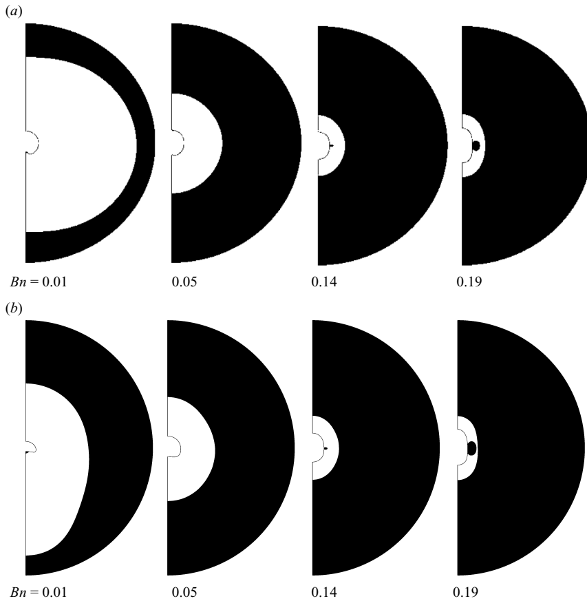
FIGURE 9. Dependence of the bubble shape and the yielded (white) and unyielded (grey) domains on Bn for N = 10^4 and (a) Ar = 1 , Bo = 50 , (b) Ar = 50 , Bo = 10 , for Bn = 0.01 , 0.05 , 0.14 , and 0.19 ; R_\infty = 10 in all cases except for the first one in (b) where R_\infty = 15 .
